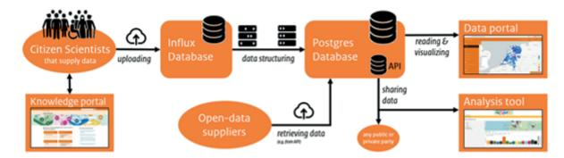
Figure 8: Diagram of the Measure Together infrastructure.
