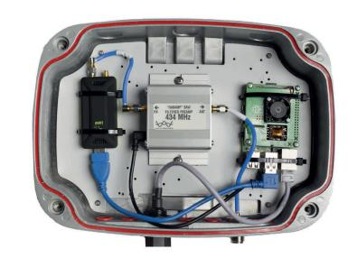
Figure 13: View of interior of ground station transceiver. Source: LSTN Handbook
